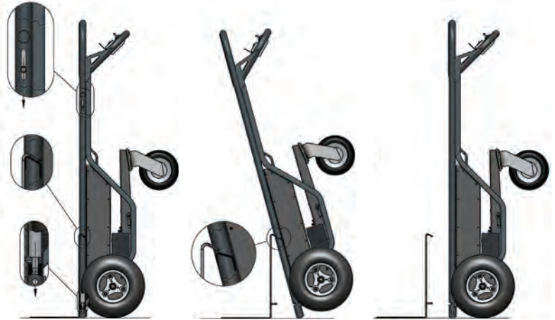
Capture/Release by Leaning Truck Forward and Pulling Release Handle.
