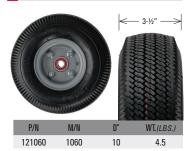
4-ply tube-type tire with three-piece off-set hub and semi-precision bearings.
